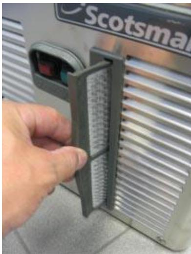
Pull out the removable condenser air filter on the front of the machine, vacuum to clean or wash in clean water and dry, refit it in to the runner moulding once complete.
