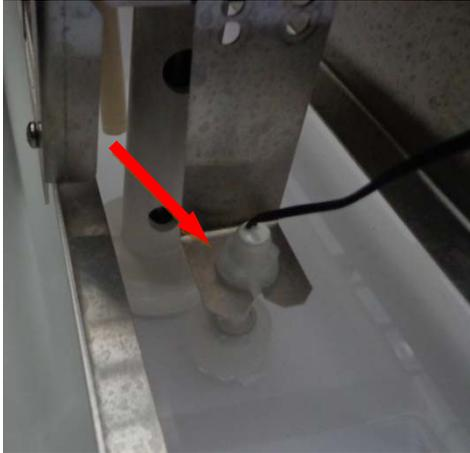
The water level sensor is located at the top of the water tank. When water level reaches a certain level during water filling, the magnetic sensor of the water level sensor detects the magnetism and signals it to the PC board. Once the PC board receives the signal, then it will power off the water inlet valve and water filling is stopped.
