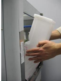
On the MC Range remove the plastic sump cap of the sump to drain the unit
