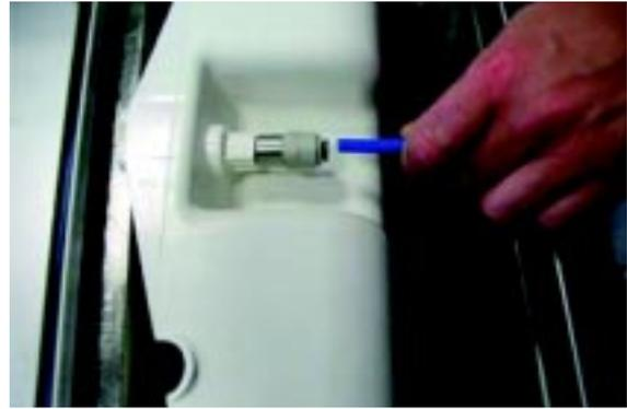
.....and remove water sump from evaporator basin
