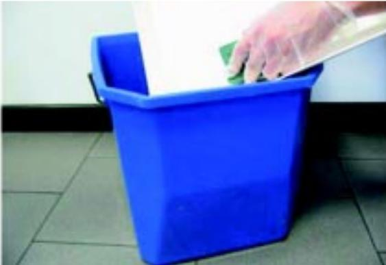
14. Once reservoir is duly cleaned, dump float valve in the solution and remove any kind of scale or mineral deposit then rinse the same by fresh water.
