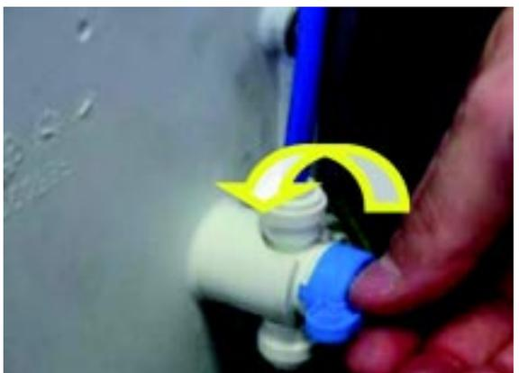
5. Bend down the plastic hose and drain out the water from the water sump then move it up again.
