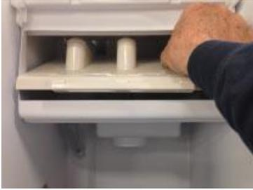
7. Using a container, pour water into the bottom of the sump/freezing chamber to rinse out most of any loose scale deposit.
