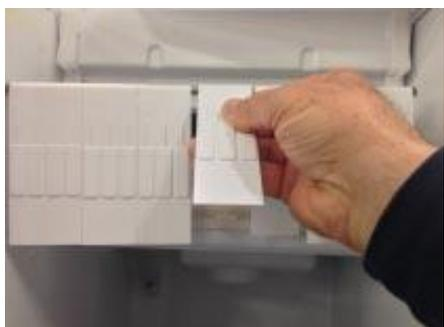
6. Lift up the entire spray platen, disconnect water hose and take it out to clean the water jets separately
