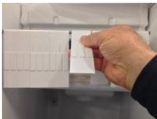
14. Pour over the evaporator two or three litres of clean potable water to rinse the evaporator platen.
