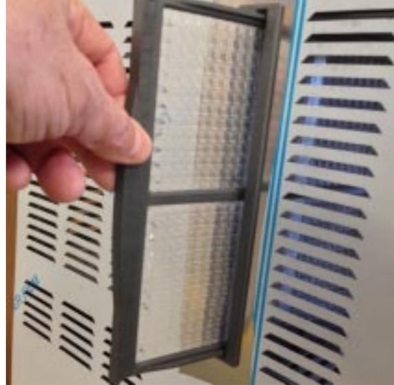
2. Blow pressurised air on the opposite direction of the condenser air flow so to remove the dust accumulated.
